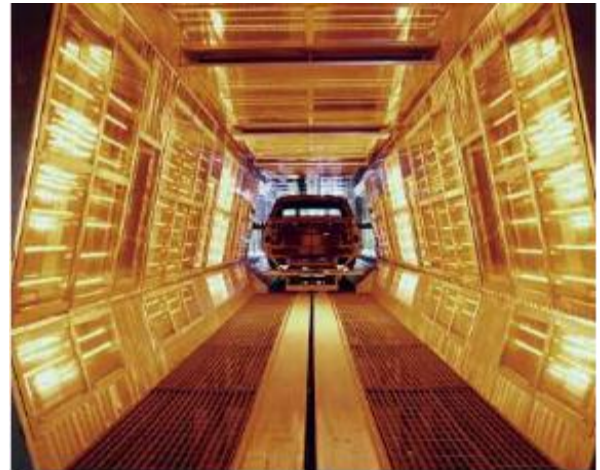
Figure 6. Modern nanocoatings and special nanopaints can be successfully dried or hardened with infrared heat.
