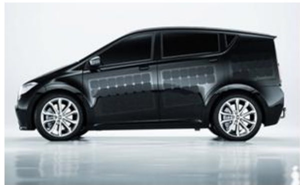
Figure 7. The Sion is the first electric car capable of recharging its batteries from the sun.
